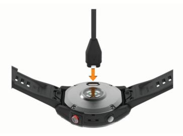
**2** Plug the other end of the cable into a USB charging port. The watch displays the current battery charge level.
